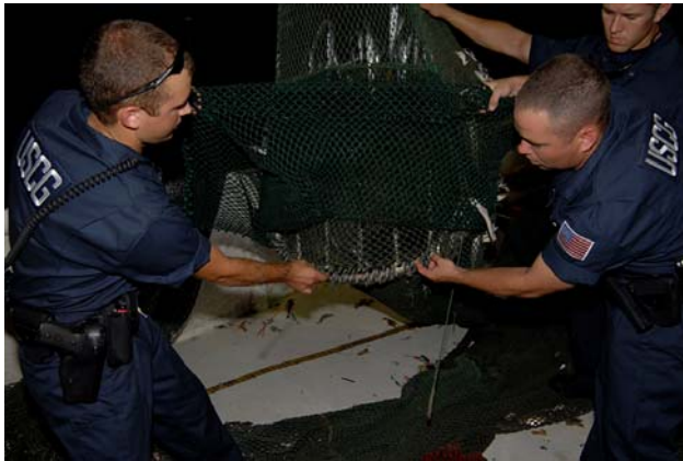
GULF OF MEXICO - Resolute boarding officers inspect the skirt on a shrimp net placed above the TED. The net's escape chute was sewn shut, shown here as the lighter green net, and a darker green false skirt was sewn over it to make the TED appear functional. The chutes above the TEDs must remain open to allow sea turtles to be ejected from the net. Coast Guard photograph by PA3 Rob Simpson.
